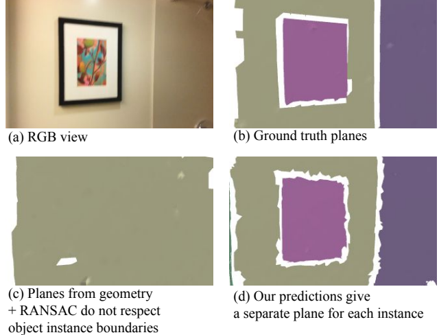
Figure 5. Sequential RANSAC alone is not enough to segment planar instances. Sequential RANSAC (with geometry from [58]) does well, but fails to segment adjacent co-planar instances. Our method can segment these, e.g., this picture frame.
