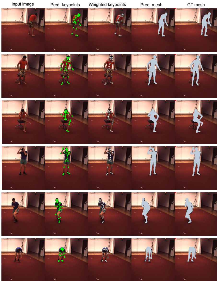
Fig. 8: Human3.6M: Camera-space full body mesh qualitative results on test images. We observe that our method can also be used in the problem of camera-space full body mesh prediction. Interestingly, we note that the method tends to assign higher weights to the keypoints in the head, feet, and torso-pelvis, which are likely to be less occluded or variable compared to, for example, the arms and hand.
